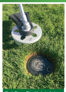
Each Power Trim blade includes a 1" Arbor hole and 20mm bushing for ECHO brand trimmers
